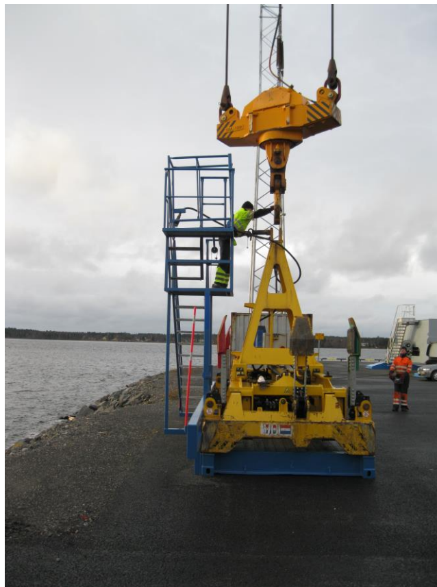
VDL spreader attached to mobile crane hook beam
