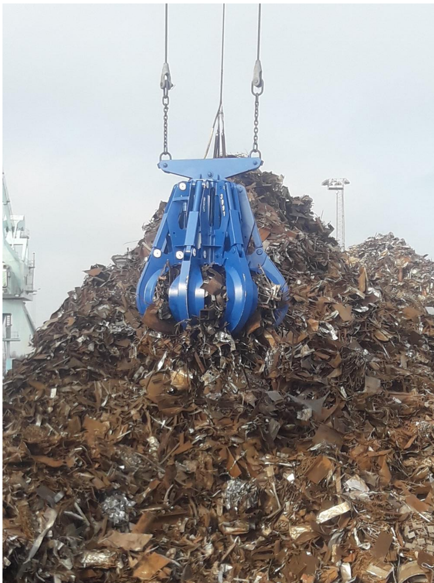
6 m 3 Orange peel motor grab operating at Associated Danish Ports A/S in Fredericia
