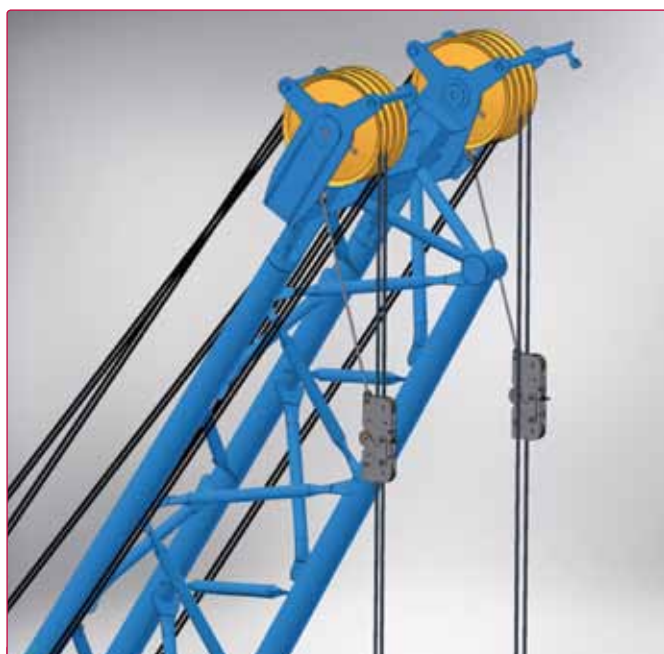
Rope inclination sensors fitted to the boom tip automatically guarantee the hook is positioned exactly vertically over the load.
